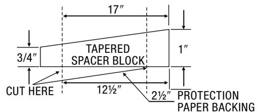
4. The 2½" section is placed in front of the rib on base with the tapered end facing the back of the sleeve. Cut the remaining portion to 12½" and place behind the rib again, sloping toward the rear of the sleeve. This helps to induce a rearward slope on the unit.
