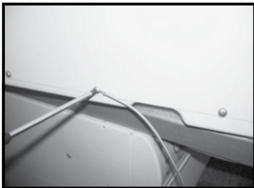
1. Remove existing rear grille and replace with provided louvered panel. Install as shown here.
