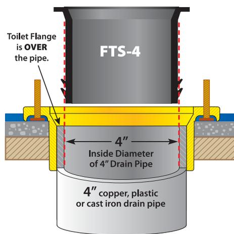
The **FTS-4** Wax Free Toilet Seal seals to the 4" inside diameter of 4" plastic, copper or cast iron drain pipe on both floor mounted and back outlet toilets. Including smooth wall 4" wall carrier models.
