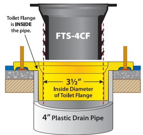
The **FTS-4CF** Wax Free Toilet Seal seals to the 3 1/2" inside diameter of plastic toilet flanges installed inside 4" plastic drain pipe. These flanges are sometimes referred to as a Combination Flange, Slab Flange, or 4x3 Flange.
