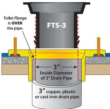
The **FTS-3** Wax Free Toilet Seal seals to the 3" inside diameter of 3" plastic, copper or cast iron drain pipe.
