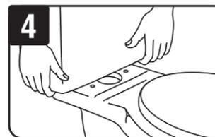
Before replacing the tank on the bowl, place metal washer and hex nut onto bolt under tank and hand tighten hex nut. Then place tank back on the bowl gasket so that tank to bowl gasket fits evenly. Level tank. Under the bowl attach rubber washer, metal washer and metal hex nut. Tighten the hex nuts under the bowl evenly until the tank is stable and doesn't rock. **DO NOT OVERTIGHTEN** or the tank or bowl could break.
