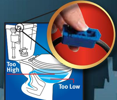
The refill adjuster allows the right amount of water to be delivered to the bowl. Too high a refill to the bowl wastes water down the drain. Too low can cause an improper flush or sewer gas to leak into the room.
