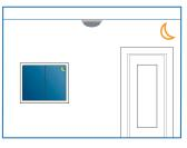
3. If no presence is detected the light dims to 10%/20%/30%/50% (options) stand-by levels after the hold time.
