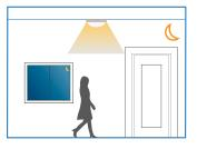
2. With insufficient natural light, the light is switched on automatically when presence is detected; it will remain on 100% during the motion hold-time.
