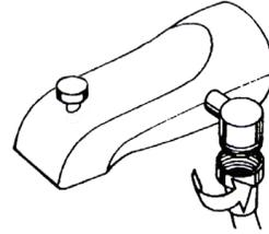
The diverter outlet on the side of the spout is for a hose connection to operate a hand shower. Use either end of the flexible hose. Hand tighten the hose nut onto the spout diverter outlet.
