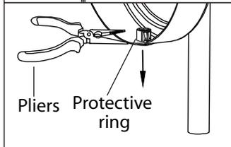
3. Use the pliers to remove the protective ring.
