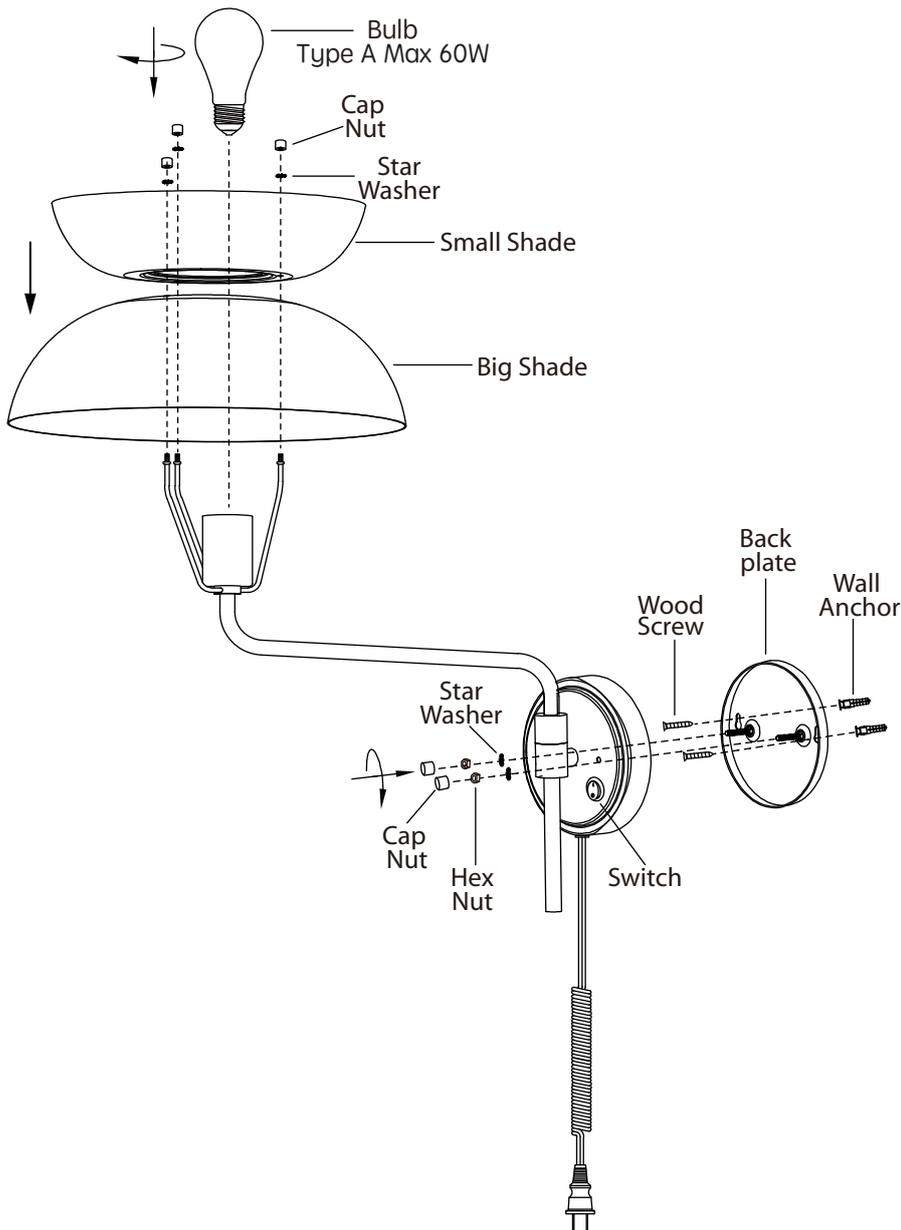
1. Remove the back plate from the fixture by unscrewing cap nuts, hex nuts and star washers.
