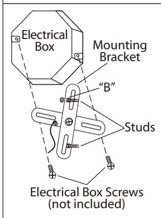
5. Loosen "B". Adjust stud to desired length and lock in place with "B". Mount the mounting bracket to electrical box using electrical box screws. Make sure the studs on the mounting bracket are facing out from the electrical box.
