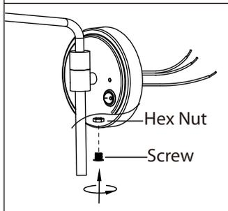
4. Fill the outlet hole by the hex nut and screw.
