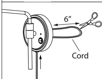
2. Use a pair of sharp scissors to cut the cord. Strip 7mm from the 6" cord.
