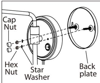
1. Remove the back plate from the fixture by unscrewing cap nuts, hex nuts and star washers.
