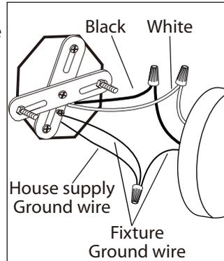
7. Connect the ground wires (bare copper or green) from the fixture to the ground wire (bare copper or green) or ground screw in the electrical box. Connect the black wire (or wire marked "SPT-2") from fixture to the black wire in the electrical box and connect the white wire (or the wire with ribbed side) from fixture to the white wire in the electrical box.
