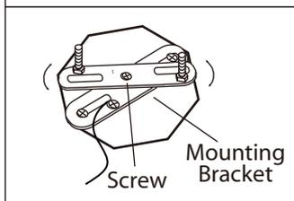
6. Position mounting bracket so that the fixture will be hung properly once it is mounted to the ceiling. Tighten the screw to hold in place.
