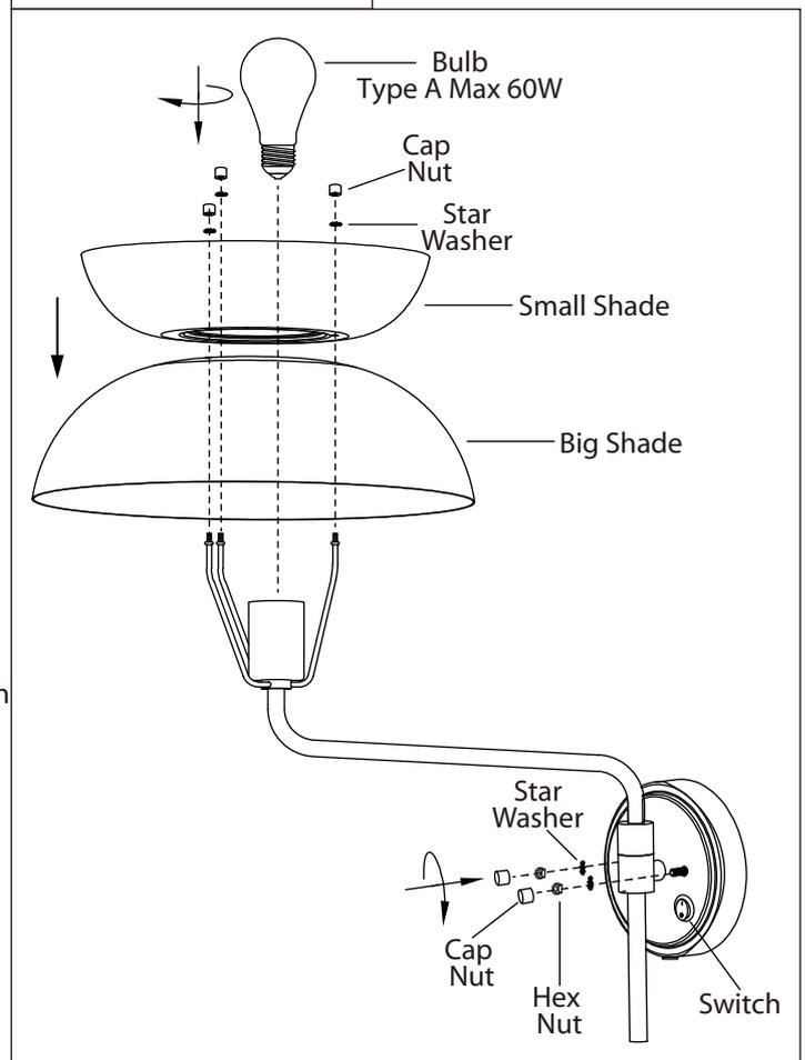
9. Position fixture over studs on mounting bracket assembly. Secure fixture in place with the star washers, hex nuts and cap nuts.
