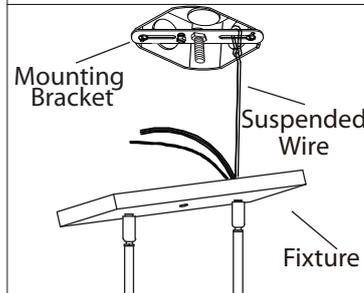
7. Use the suspended wire to hang the fixture as shown for wiring connection.
