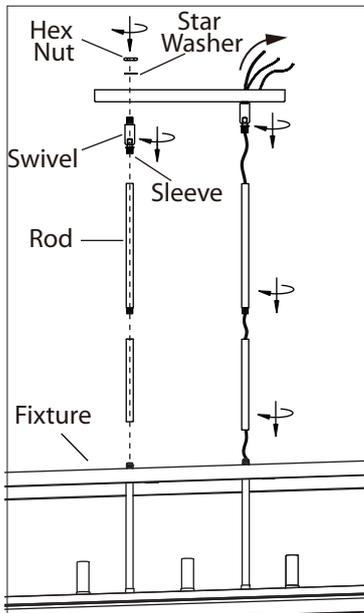
4. Position the covers in place. Install the length of rod that is required by threading wire through the rod and screwing it to the fixture. Install swivel to the rod, ensuring that the sleeve is at the swivel.
