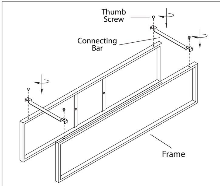
1. Remove the thumb screws that are already on the frames. Position the frames as shown. Install the 4 connecting bars on to the frames by tightening the thumb screws.
