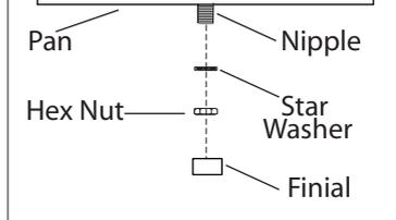
10. Secure the pan to the nipple tightening by star washer and hex nut. Screw the finial to the nipple.
