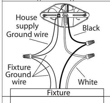
8. Connect the ground wires (bare copper or green) from your fixture to the ground wire (bare copper or green) or ground screw in the electrical box. Connect the black wire from the fixture to the black wire in the electrical box and connect the white wire from the fixture to the white wire in the electrical box.
