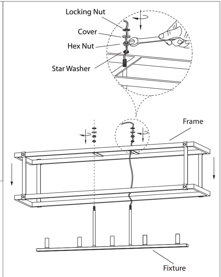
2. Remove the locking nuts, covers, hex nuts and star washers from the fixture. Feed the wires from the fixture through the holes in the frame and position the fixture into the frame as shown.
