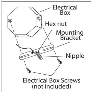
6. Attach nipple to mounting bracket. Adjust so it will clear hole in back of fixture and then lock nipple in place with star washer and hex nut. Attach mounting bracket to electrical box with electrical box screws (not included).
