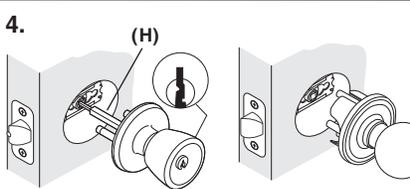
**5. INSTALL INTERIOR ASSEMBLY.** Interiors must be in locked position on Entry and Bed/Bath functions before installing.
