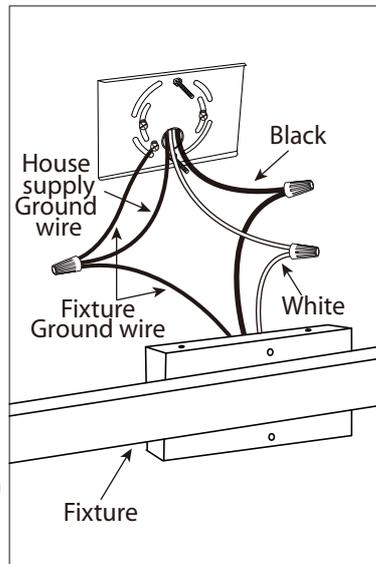
3. Connect the ground wires (bare copper or green) from your fixture to the ground wire (bare copper or green) or ground screw in the electrical box. Attach the black wire from the light fixture to the black wire in the electrical box. Attach the white wire from the light fixture to the white wire in the electrical box.
