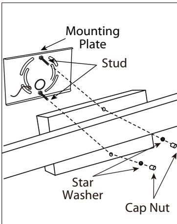
1. Remove the mounting plate from the fixture by unscrewing the cap nuts and star washers.
