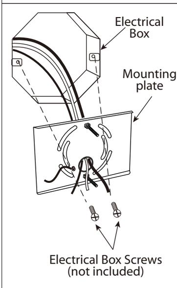
2. Feed power cords from the electrical box through the centre hole of the mounting plate. Align holes of mounting plate over electrical box and secure with electrical box screws (not included).
