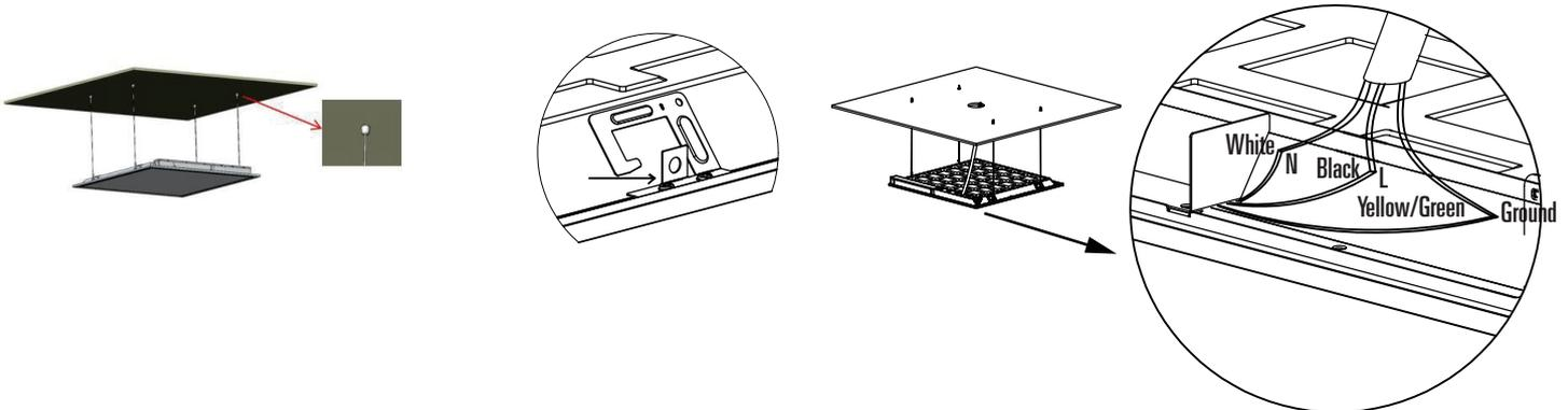
2. With power turned off at the breaker, connect power to driver based on the wiring diagram to complete the installation.
