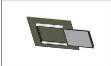
3. Slide luminaire partially into mounting frame as shown. With power turned off at the breaker, connect power to driver based on the wiring diagram.
