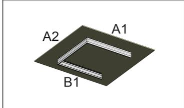
2. Attach the frame to the ceiling with screws (using approved anchors). Remove frame piece B2 as shown in picture 1.
