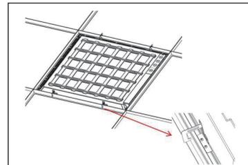
3. Fold the 4 protection brackets so they will be above the T-bar as shown.
