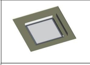
4. Slide luminaire fully into frame as shown.
