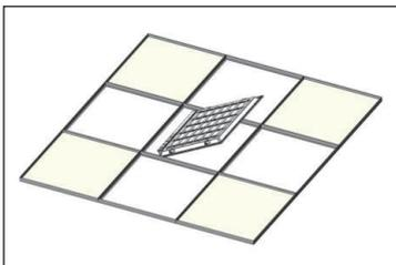
1. Remove the ceiling tile at an appropriate location where the product is to be installed and raise the product above the bar.
