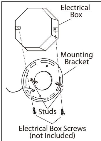
1. Mount the mounting bracket to outlet box using electrical box screws (not included). Make sure the studs on the mounting bracket are facing out from the electrical box.
