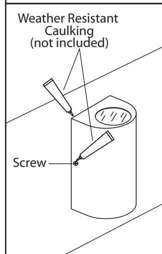
5. After installation, seal around the top and side perimeter between the fixture and the wall surface with weather resistant caulking. The bottom should be left un-caulked to prevent moisture build-up. Apply a small amount of weather resistant caulking around the side perimeter between the screw and mounting plate.
