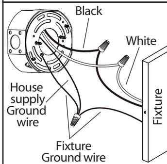
2. Connect the ground wires (bare copper or green) from your fixture to the ground wire (bare copper or green) or ground screw in the electrical box. Connect the black wire from the fixture to the black wire in the electrical box and connect the white wire from the fixture to the white wire in the electrical box.
