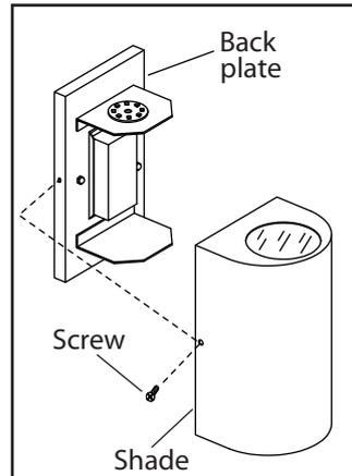
4. Attach the shade to the back plate by tightening the 2 screws.
