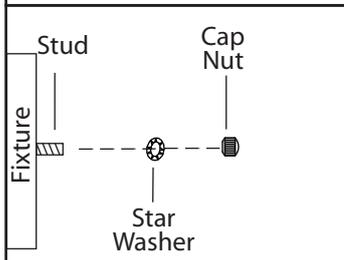
3. Once connections of wires are completed, carefully tuck wires and wire nuts into the electrical box making sure no bare wire is visible at the wire nuts. Install the light fixture to the wall by aligning the holes in the fixture with the studs on the mounting bracket. Secure in place with cap nuts and star washers.
