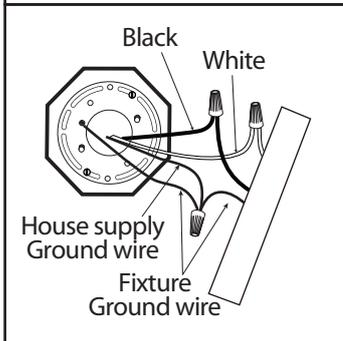
2. Connect the ground wires (bare copper or green) from your fixture to the ground wire (bare copper or green) or ground screw in the electrical outlet box. Connect black wire from fixture to black wire in outlet box and connect the white wire from fixture to white wire in outlet box.
