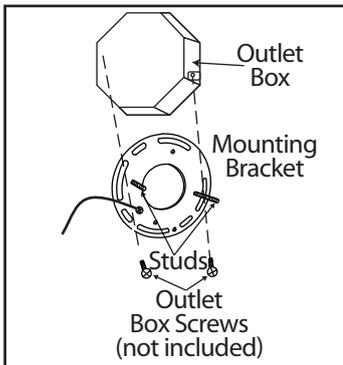
1. Mount the mounting bracket to outlet box using outlet box screws (not included). Make sure the studs on the mounting bracket are facing out from the outlet box.
