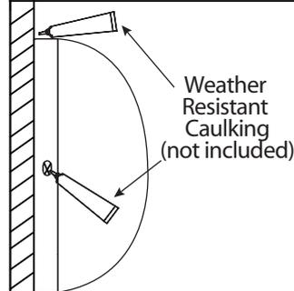
5. After Installation, seal around the top and side perimeter between the fixture and the wall surface with weather resistant caulking. The bottom should be left un-caulked to prevent moisture build-up. Apply a small amount of weather resistant caulking around the side perimeter between the cap nut and mounting plate.
