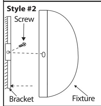
**Style #2** Attached fixture to mounting bracket by tightening the 2 screws.
