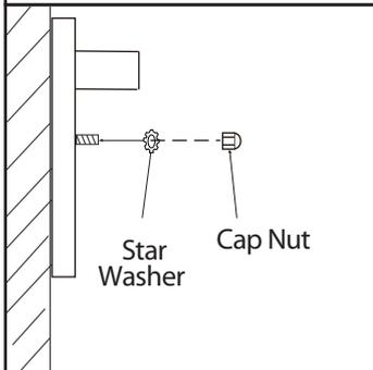
3. Once connections of wires are completed, carefully tuck wires and wire nuts into the outlet box making sure no bare wire is visible at the wire nuts. Install the light fixture to the wall by aligning the hole(s) in the fixture with the studs on the mounting bracket. Secure in place with cap nut(s) and star washer (s).
