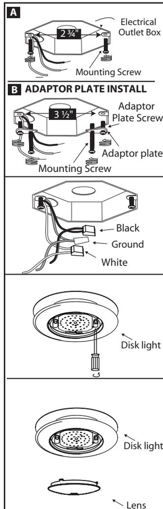
1. Prior to installation you will need to determine if the electrical box requires the adaptor plate. If the distance between the mounting screws in your electrical outlet box is greater than 2 3/4" you will need to use the adaptor plate. Securely tighten adaptor plate, with adaptor plate screws. Do not drive mounting screws completely to the end of the junction box.
