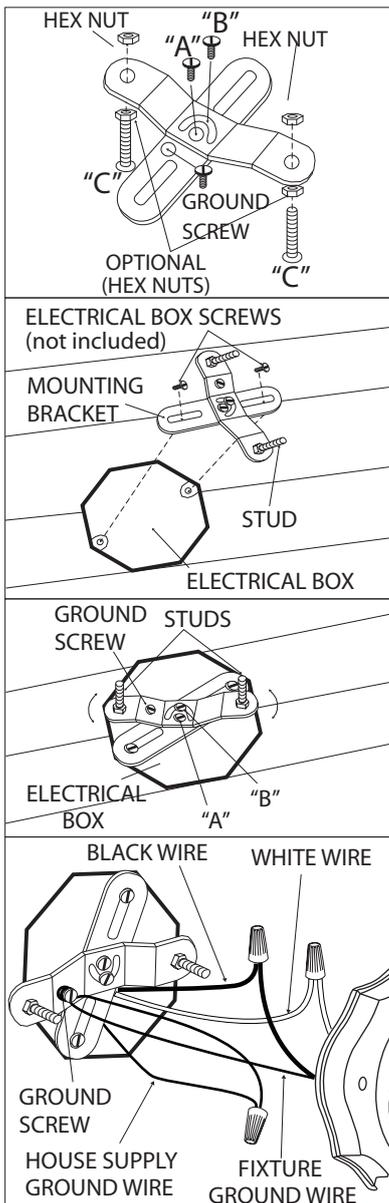
1. Assemble the mounting bracket (2 pieces) as per drawing. "A" and "B" screws should only be snug at this point. Screw "C" may be tightened and locked in place with hex nut(s) (if mounting bracket holes are untapped, an additional two hex nuts are required). The ground screw should then be attached to the mounting bracket (do not tighten).
