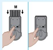
The Status LED will flash red and green, and the lock will beep. Press and release the Program button again. The latch bolt will retract and extend on its own.
