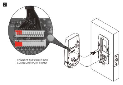
Note: The metal connector side should face outside.
