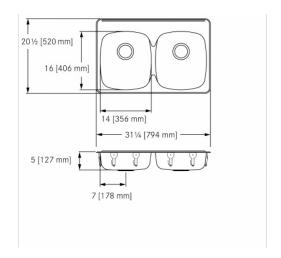
Double compartment self rimming drop-in sink with faucet ledge. 18 gauge (1.2 mm), type 304 (CNS 18/10) stainless steel. Exposed surfaces are #4 satin finished. Undercoated to reduce condensation and resonance. Includes waste fittings, factory applied rim seal, cutout template, and factory installed EZ TORQUE™ fasteners. Certified to ASME A112.19.3-2008 / CSA B45.4-08.
