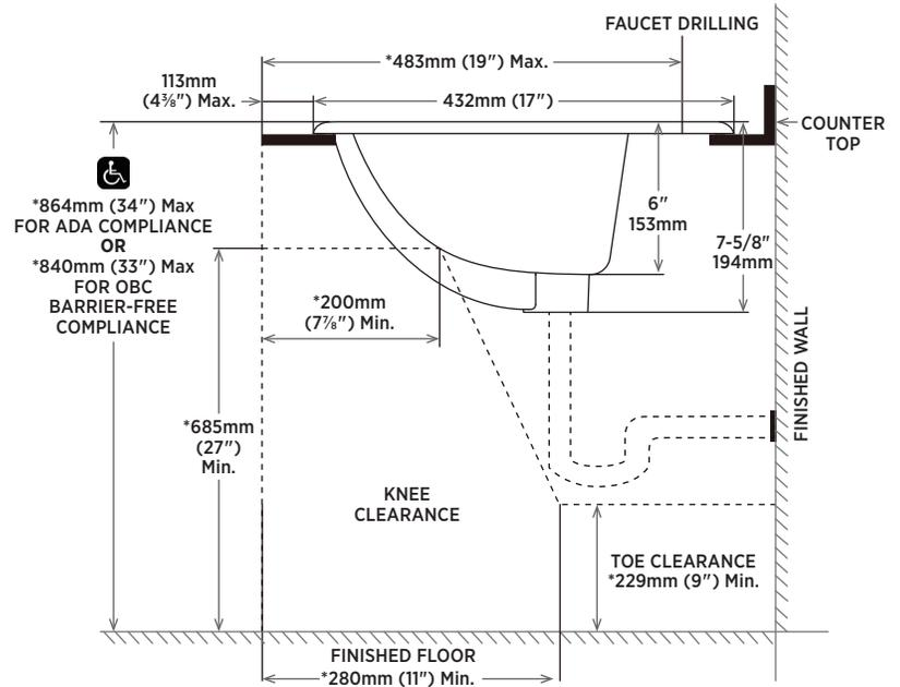
**NOTE:** \* Starred measurements comply with ADA and OBC barrier free accessibility requirements. ▲ Dimensions shown for location of supplied and waste are suggested.
