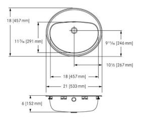
Single compartment self rimming vanity basin with faucet ledge. 18 gauge (1.2 mm), type 304 (CNS 18/10) stainless steel. Mirror finished rim, #4 satin finished bowl. Undercoated to reduce condensation and resonance. Includes factory applied rim seal, cutout template, and installation hardware. Certified to ASME A112.19.3-2008 / CSA B45.4-08.
