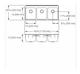
Triple compartment self rimming drop-in sink with faucet ledge. 18 gauge (1.2 mm), type 304 (CNS 18/10) stainless steel. Exposed surfaces are #4 satin finished. Undercoated to reduce condensation and resonance. Complete with waste fittings, factory applied rim seal, and factory installed EZ TORQUE™ fasteners. Certified to ASME A112.19.3-2008 / CSA B45.4-08.
