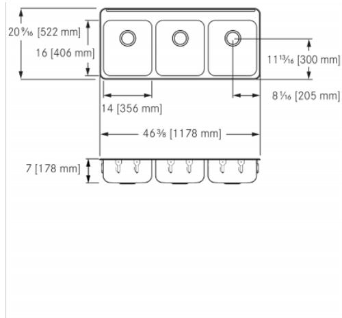
Triple compartment self rimming drop-in sink with faucet ledge. 20 gauge (0.9 mm), type 302 (CNS 18/8) stainless steel. Exposed surfaces are #4 satin finished. Undercoated to reduce condensation and resonance. Complete with waste fittings, factory applied rim seal, and factory installed EZ TORQUE™ fasteners. Certified to ASME A112.19.3-2008 / CSA B45.4-08.
