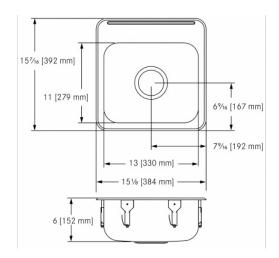
Single compartment self rimming drop-in sink with faucet ledge. 20 gauge (0.9 mm), type 302 (CNS 18/8) stainless steel. Exposed surfaces are #4 satin finished. Undercoated to reduce condensation and resonance. Includes waste fitting, factory applied rim seal, cutout template, and factory installed EZ TORQUE™ fasteners. Certified to ASME A112.19.3-2008 / CSA B45.4-08.
