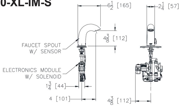
NOTE: Recommended through hole diameter to properly mount the spout/shank is 1-1/8" to 1-1/4".
