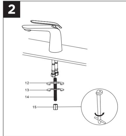
2. From under the sink secure the faucet with fixing kit (12), (13), (14), (15).
