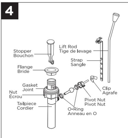
4. (if applicable remove the old pop-up drain and clean the hole in preparation for the new pop-up drain installation). Remove the stopper and flange.
