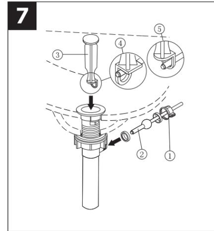
7. Remove pivot nut (1). Install horizontal rod (2) and stopper (3) as removable (4) or non-removable (5). Hand tighten pivot nut (1).
