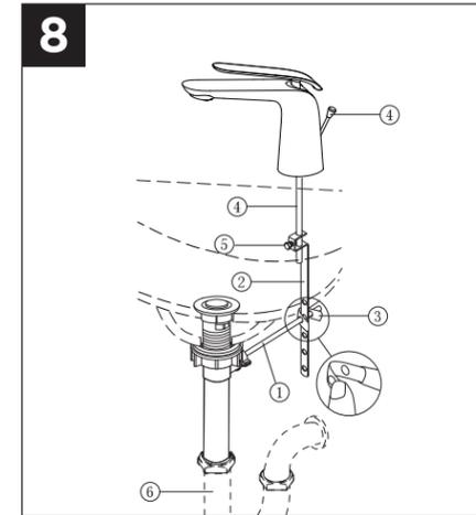
8. Attach horizontal rod (1) to strap (2) using clip (3). Install lift rod (4), tighten screw. Connect assembly to drain (6).
