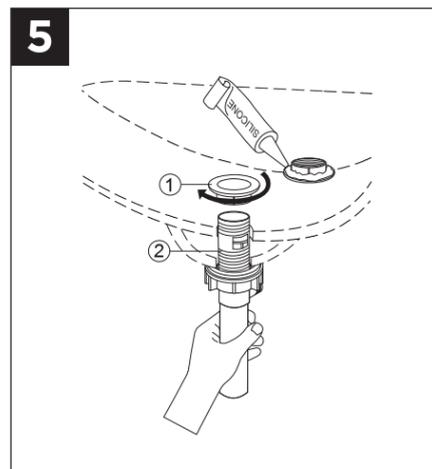
5. From under the sink insert the pop-up drain through the hole of basin. Apply silicone to underside of the flange (1) and screw it into the body of pop-up drain (2).
