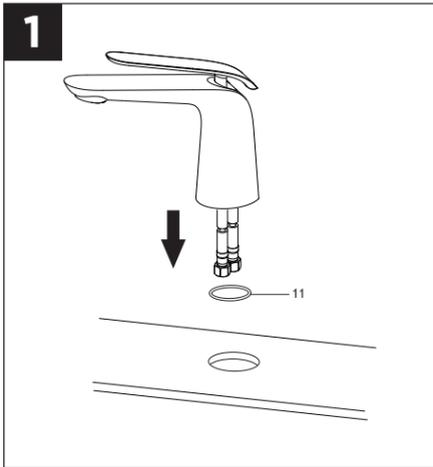
1. Shut off water supplies. Place new faucet through hole(s) in top of sink using (11) O-Ring.
