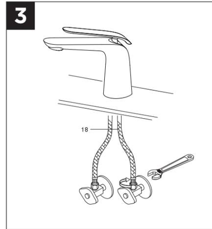
3. Connect the hot and cold water supply lines (18) to the angle stop (not included). Use wrench as shown. **Caution: Do not overtighten.**
