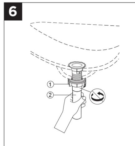
6. Adjust the pivot to face faucet, hold the tailpiece (2) and tighten the nut (1) firmly. **Caution: Do not overtighten.**
