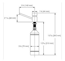
Chrome soap dispenser manufactured from chromium plated brass. Incorporates a replaceable 1 litre polyethylene container for use with liquid soap standard. Support rod fits 7/8" to 1 1/4" (22 - 32 mm) opening.
