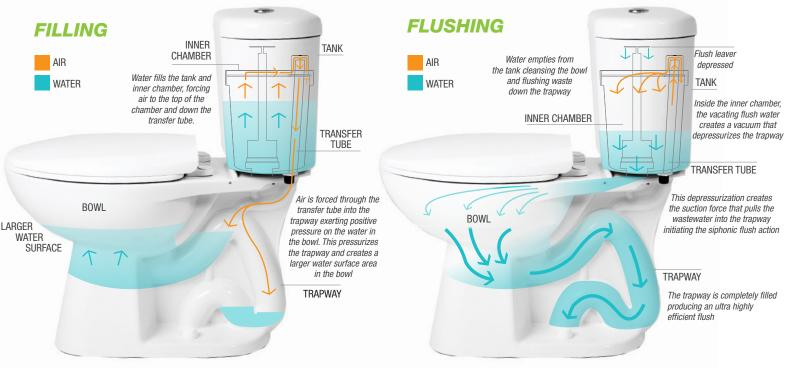
With an innovative technique, H & H have revolutionized the toilet flush. By harnessing the energy created by water filling the tank, Proficiency uses a patented air transfer system to pressurize the trapway. Once activated, the swift and powerful flush evacuates all waste in the bowl.
