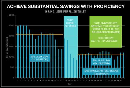
Daily water consumption at St. David's Towers in Toronto, before and after installation of Proficiency UHET
