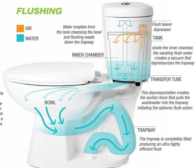
With an innovative technique, H & H have revolutionized the toilet flush. By harnessing the energy created by water filling the tank, Proficiency uses a patented air transfer system to pressurize the trapway. Once activated, the swift and powerful flush evacuates all waste in the bowl.
