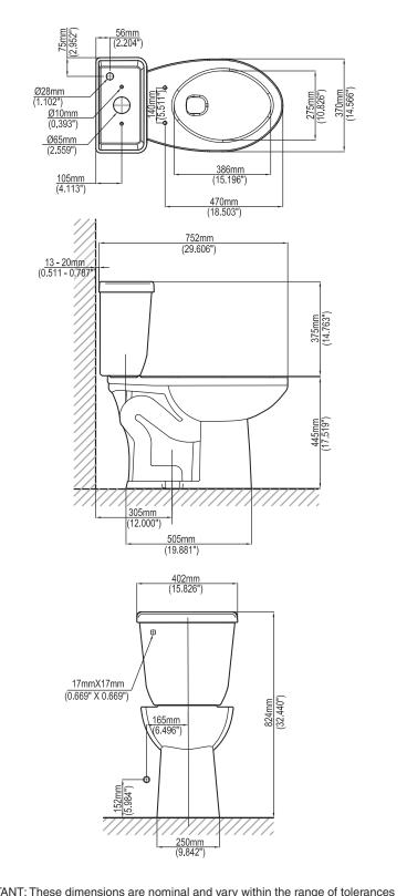
IMPORTANT: These dimensions are nominal and vary within the range of tolerances established by ASME standard A112.19.2.
