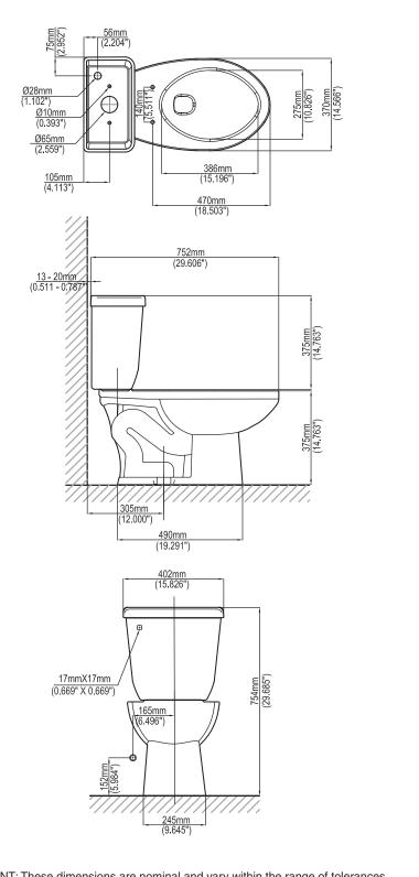
IMPORTANT: These dimensions are nominal and vary within the range of tolerances established by ASME standard A112.19.2.
