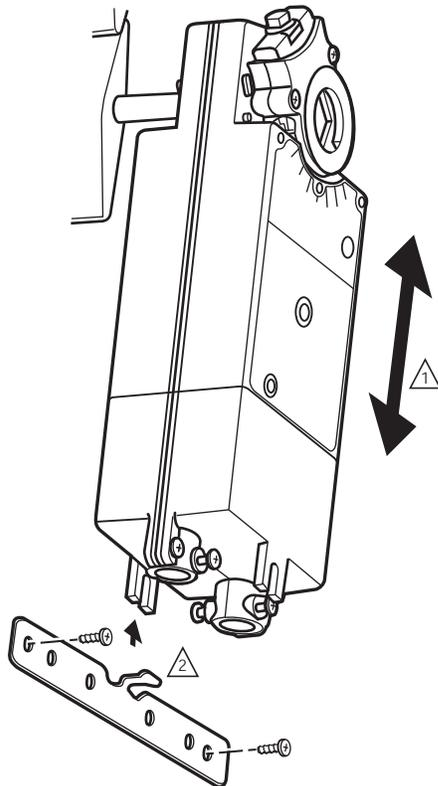
1 ENSURE THAT MOUNTING ASSEMBLY PREVENTS ACTUATOR ROTATION AND ALLOWS ACTUATOR TO FLOAT ALONG INDICATED AXIS. WHEN TOO TIGHT, THE RESULTING BINDING CAN DAMAGE THE ACTUATOR OR REDUCE TORQUE OUTPUT.
