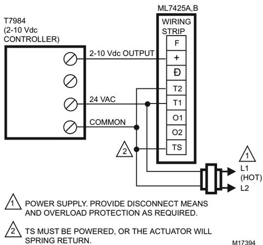
Fig. 8. ML7425 Wiring.
