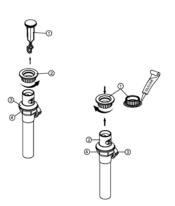
Apply silicone to underside of flange (#1). Insert body (#2) into sink. Screw flange onto body. Pivot hole (#3) must face back of sink. Tighten nut/gasket (#4), clean off
