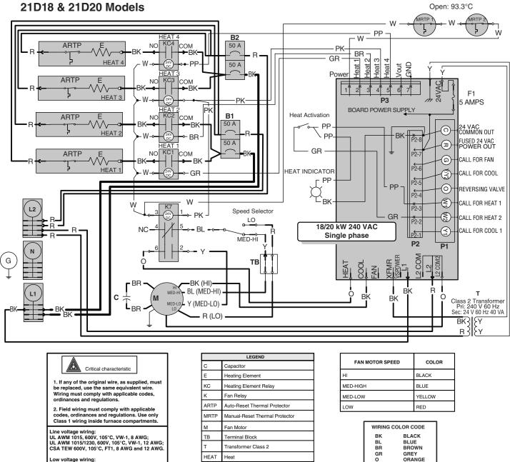
Low voltage wiring: same ratings as high voltage except 18 AWG.
