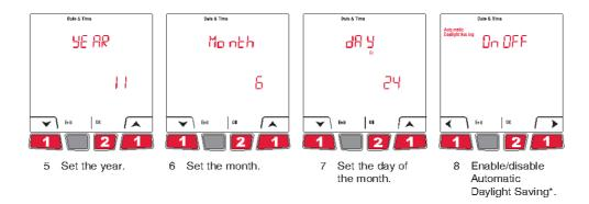
\* When this function is enabled, the thermostat switches to daylight savings time on the second Sunday of March and to normal time on the first Sunday of November. When the function is disabled, the thermostat keeps the normal time all year long.
