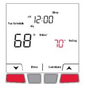
Press ▲ or ▼ until the desired temperature is displayed.
