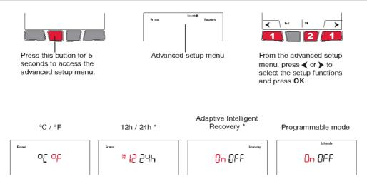
\* These parameters are available only if the thermostat is configured in programmable mode.
