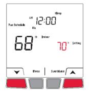
Press ▲ or ▼ until the desired temperature is displayed.
