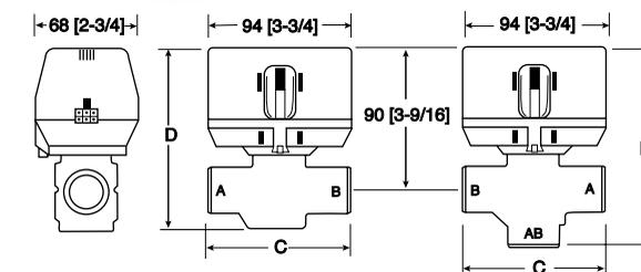
Figure 1 - Nominal dimensions in inches and millimetres
