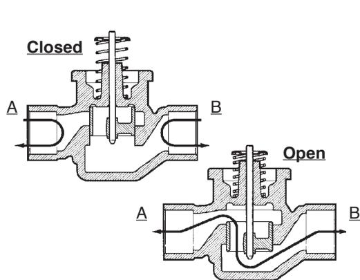
Figure 2 - Fluid flow of 2-way valves
