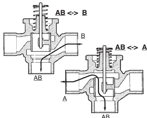
Figure 3 - Fluid flow of 3-way valves
