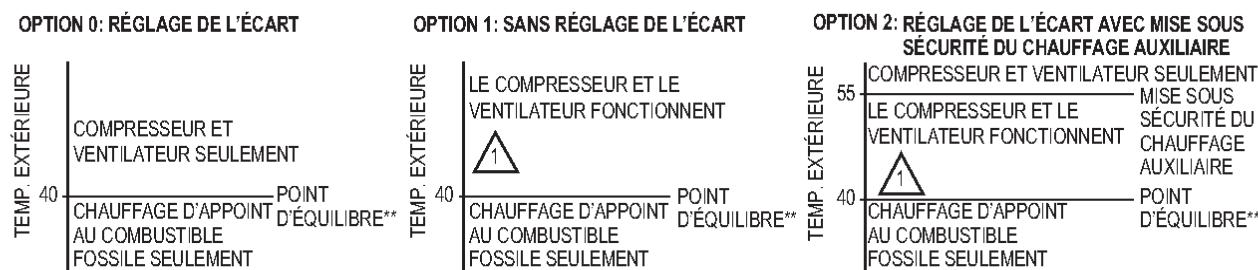
**⚠** SI LA TEMPÉRATURE AMBIANTE BAISSE (DÉPASSEMENT DU RÉGLAGE DE L'ÉCART À LA FONCTION 20), LE COMPRESSEUR EST DÉSACTIVÉ. LE CHAUFFAGE D'APPONT AU COMBUSTIBLE FOSSILE EST ACTIVÉ APRÈS 3 MINUTES.
