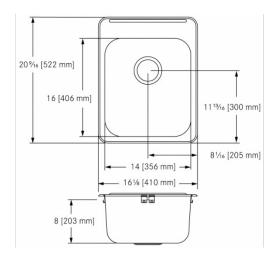
Single compartment self rimming drop-in sink with faucet ledge. 18 gauge (1.2 mm), type 304 (CNS 18/10) stainless steel. Exposed surfaces are #4 satin finished. Undercoated to reduce condensation and resonance. Includes waste fitting, factory applied rim seal, cutout template, and factory installed EZ TORQUE™ fasteners. Certified to ASME A112.19.3-2008 / CSA B45.4-08.
