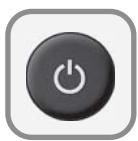
This function is ideal to perform any kind of activity in front of the sensor without operating the system (i.e. cleaning). Flushometers will remain shut for one minute when this button is pressed once. To cancel this function and to return to normal operation, press the On/Off button again or wait for function to time out.
