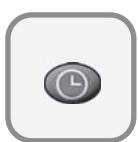
This function is used to flush urinal once every 24 hours. It also helps to prevent pipes from freezing, keeping the water moving through the pipes every 24 hours. To activate the hygiene flush, press the clock button. Wait until a quick flashing of the red light of the sensor eye is perceived. Then, press (+) to activate the hygiene flush or (-) to deactivate it.
