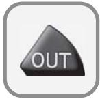
This button allows modifying the water flow time after the user removes his hands from the faucet. A delay out time close to 0 will save more water. An increased delay out time will make the user's experience more comfortable.
