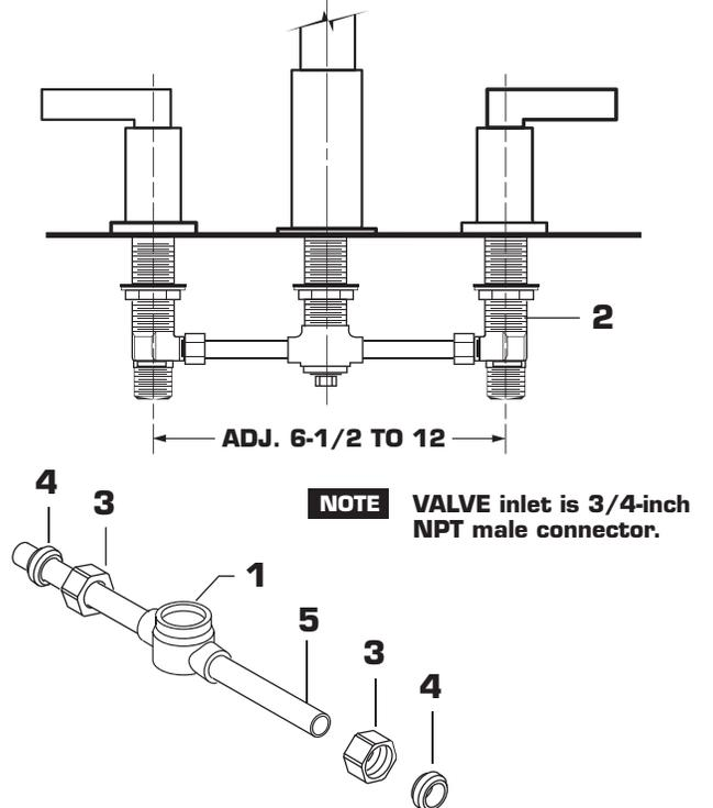
**NOTE** VALVE inlet is 3/4-inch NPT male connector.
