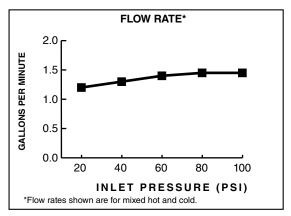
1.5 gpm/5.7 L/min. FLOW RATE
