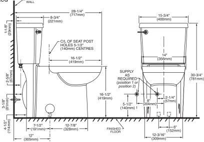
IMPORTANT: Water supply on the wall is required at 2-1/4" (57mm) or 8" (204mm) from centreline of the toilet (see rough-in). First suggested position is hidden behind the toilet. The geometry of the toilet gives space for this installation. The second suggested position is next to the toilet. Between these two positions, the space for the supply between wall and toilet is limited to 4-1/2" (114mm). In this case, check your supply and hose dimensions.
