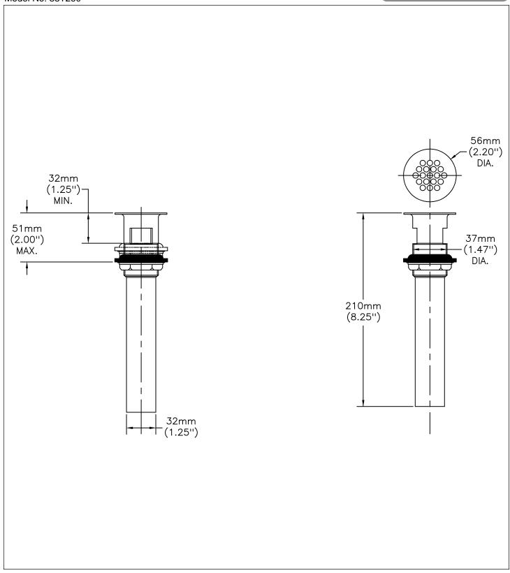
Delta reserves the right (1) to make changes to specifications and materials, and (2) to change or discontinue models, both without notice or obligation. Dimensions are for reference. Measurement may vary plus or minus 6mm(0.25"). Mounting locations are suggested only. Check with local codes for requirements in your area. This spec was produced September 10, 2018.
