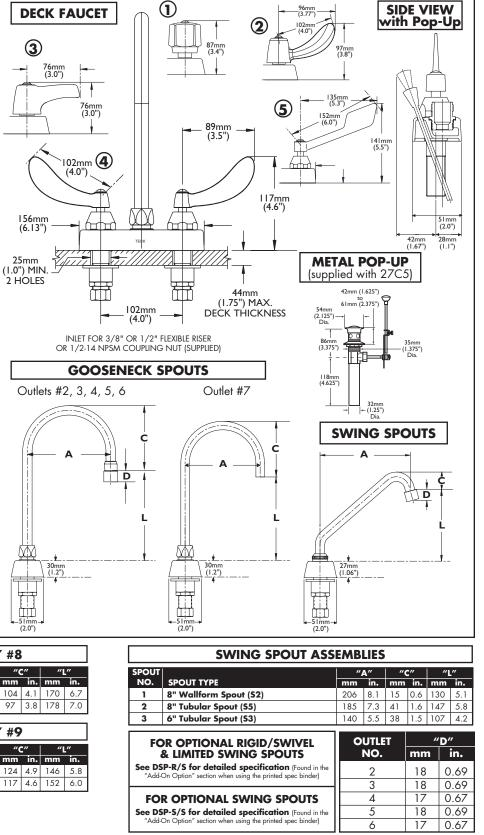
INLETS - 1/2" MIP/Coupling Nuts Note: Measurements may vary ± 6mm (0.25")
