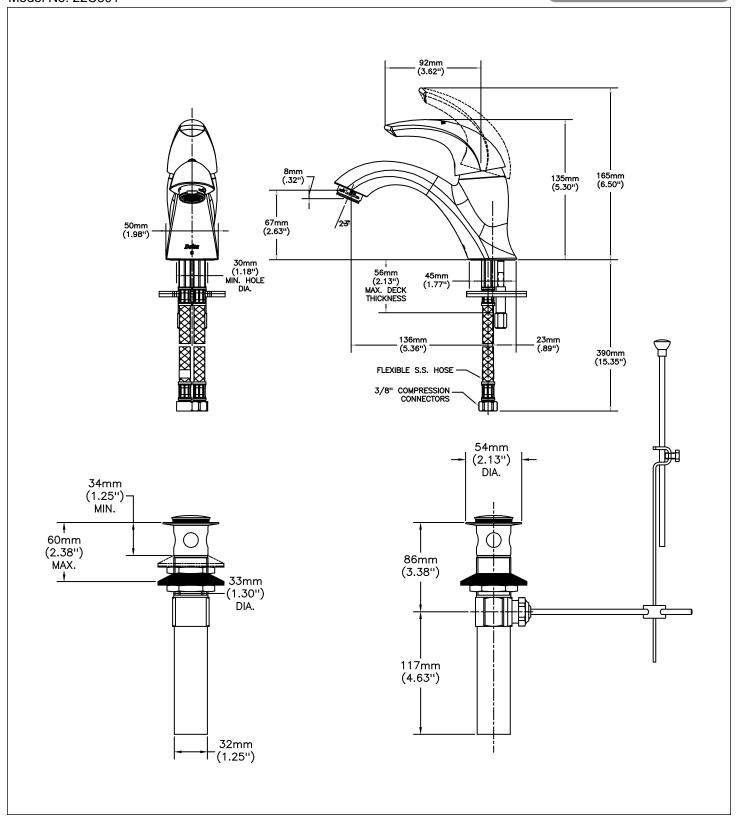
Delta reserves the right (1) to make changes to specifications and materials, and (2) to change or discontinue models, both without notice or obligation. Dimensions are for reference. Measurement may vary plus or minus 6mm(0.25"). Mounting locations are suggested only. Check with local codes for requirements in your area. This spec was produced January 29, 2013.
