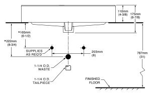
NOTES:  $\star \text{DIMENSIONS}$  SHOWN FOR LOCATION OF SUPPLIES AND "P" TRAP ARE SUGGESTED. FAUCETS NOT INCLUDED WITH FIXTURE AND MUST BE ORDERED SEPARATELY. FOR COUNTERTOP CUTOUT AND INSTALLATION INSTRUCTIONS USE TEMPLATE SUPPLIED WITH SINK.
